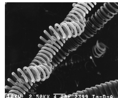
Carbon microcoils with different coil length
