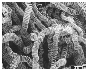
Irregularly coiled carbon microcoils with large coil diameter
