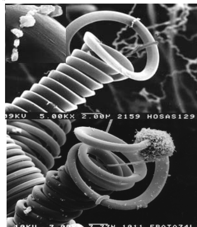
Tip Part of the carbon coil. Arrow: catalyst grain
