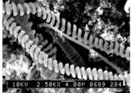
Fig. 4. Regular single-helix carbon nanocoils. Catalyst: Fe-Cr- Ni.
