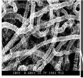
Fig. 8. Carbon microcoils with large coil diameter. Reaction temperature:  $750^{\circ}$  C, by WS<sub>2</sub> catalyst
