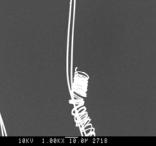
Fig. 10. Extension characteristics of carbon microcoils with big coil diameter. Recovery state after releasing the extension.
