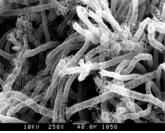
Fig. 2. Super-elastic irregular carbon coils with circular fiber cross-section and large coil diameter. Reaction temperature: 760° C, catalyst: Ni powder.
