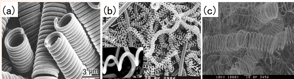
Fig. 2. SEM image of (a) typical CMCs (conventional regularly coiled CMCs) (b) SH-CMCs (c) SE-CMCs
