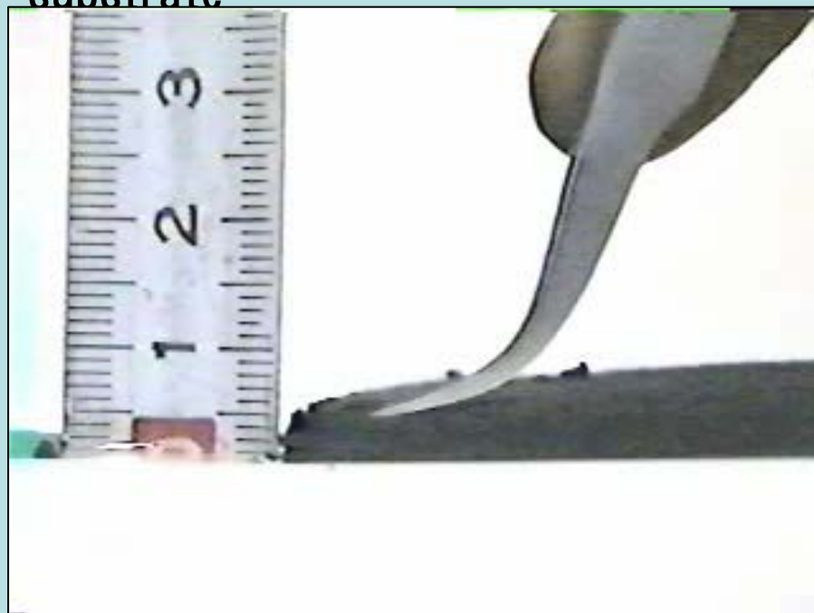
Bulk CMC as-grown on the substrate
