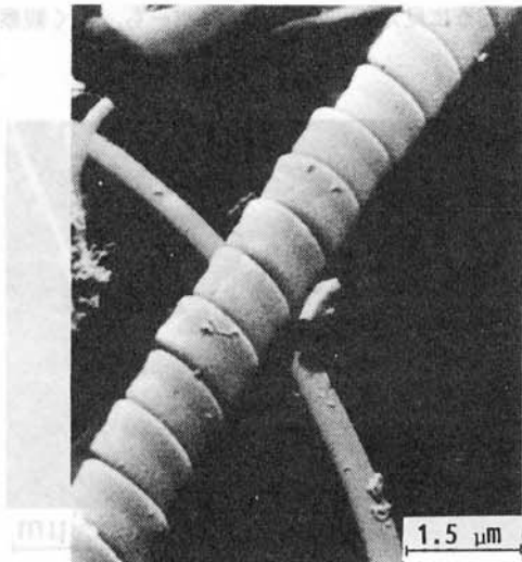
Fig. 6 Regularly coiled flat fibers (using Ni plate).
