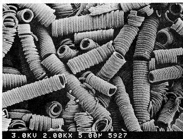
Figure 5. Ruptured short coils observed on the bottom part of the coil layers.
