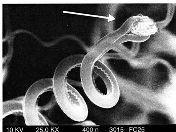
Figure 17. Interesting tip morphology of the carbon coils. Arrow indicates a catalyst grain which is a growing point.
